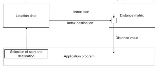
A distinction is made between main location and district in the EWS location file. Their names are in two separate columns (Name 1 and Name2). The matrix index can be different for each district, even if the postcode and the main location are identical! In the example above, note the different matrix indexes for the locations 01109 Dresden and 01109 Dresden Klotzsche. It is therefore important to also specify the district (if known) to obtain the most accurate distance between two locations.
